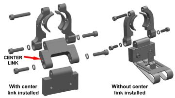
6 - The center-link may be removed if an overall shorter mount length is needed, depending on your rear view miror and desired position for the radar detector.
