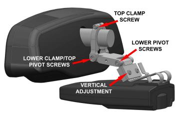
7 - Install the RD onto the mount. Make the necessary adjustments as shown above. Using the vertical adjustment, we recommend you adjust the RD as close to the bottom of the mirror as possible. The spring clip holding the RD is designed to flex downward to allow access to the RD buttons as shown below in step 9.
